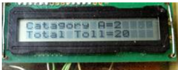
Figure 3.2 (a): Total number of vehicles and total toll collected under category A is shown in the display.
