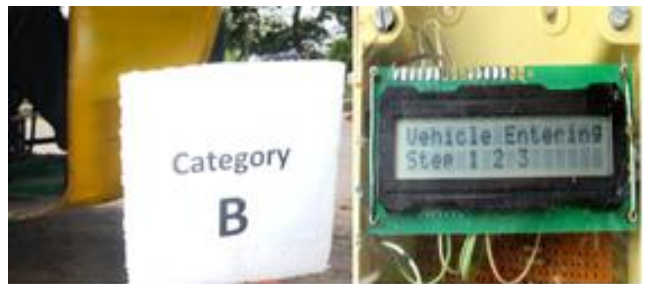
Figure 3.1 (d): Vehicle entering between 3 rd set of transmitter and receiver and step 3 is shown in the display.
