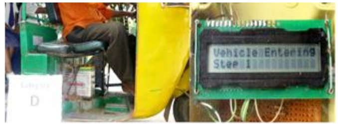
Figure 3.1 (b): Vehicle entering between 1 st set of transmitter and receiver and step 1 is shown in the display.
