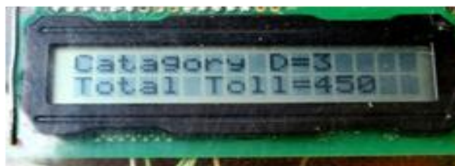
Figure 3.2 (d): Total number of vehicles and total toll collected under category D is shown in the display.
