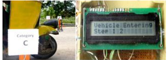
Figure 3.1 (c): Vehicle entering between 2 nd set of transmitter and receiver and step 2 is shown in the display.
