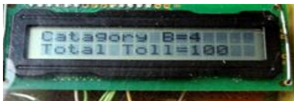
Figure 3.2 (b): Total number of vehicles and total toll collected under category B is shown in the display.
