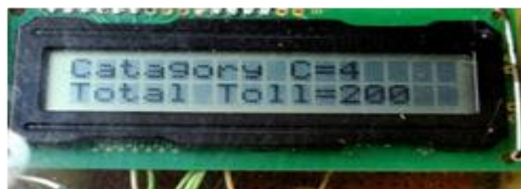
Figure 3.2 (c): Total number of vehicles and total toll collected under category C is shown in the display.
