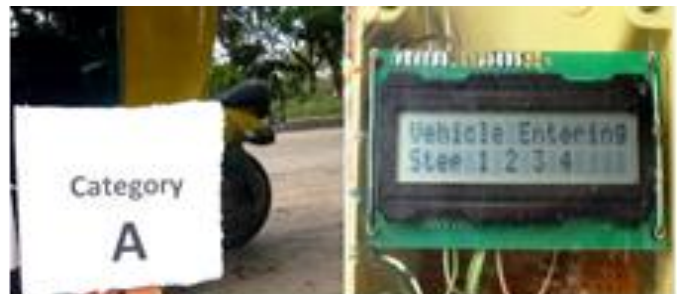
Figure 3.1 (e): Vehicle entering between 4 th set of transmitter and receiver and step 4 is shown in the display.
